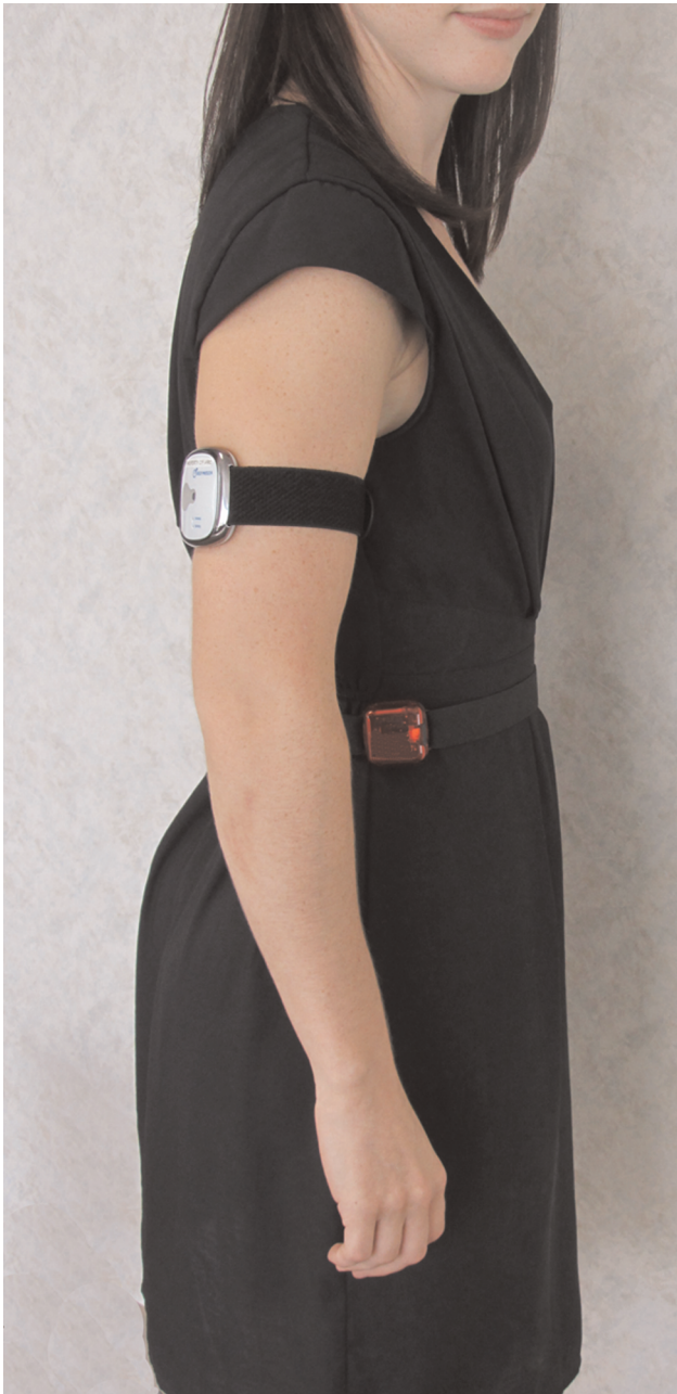
Figure 1 The SenseWear Mini (SWm) accelerometer is worn on the skin over the triceps muscle on the upper arm, and the Actigraph GT3X (AG 3 ) is worn at the waist at the mid-axillary line.
