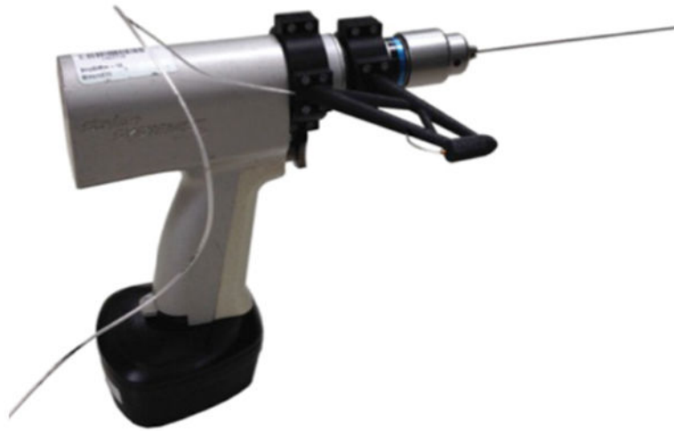
Figure 2. The electromagnetic sensors are attached to both the synthetic bone and an extension off the drill, which enables six degrees of freedom motion tracking.
