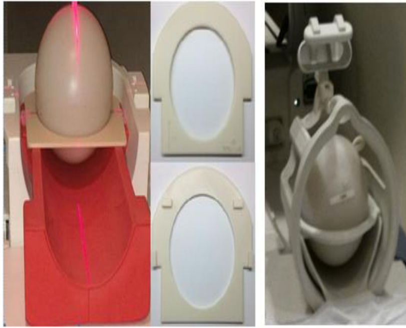
Fig. 1. Apparatus for reproducible positioning of the BIRN phantom. Left: adapter ring allowed use of standard holder for cylindrical phantoms for Siemens scanners. Center: detail of adapter rings. Right: GE scanners used standard holders for spherical phantoms.
