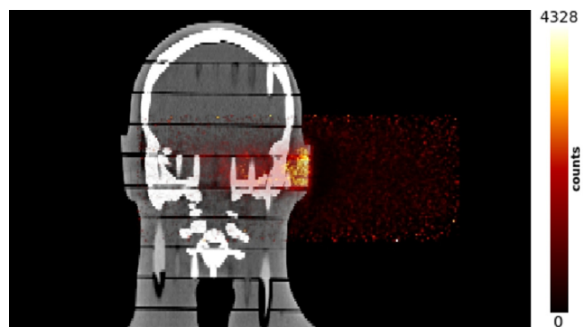
Fig. 10 Image (on the coronal view) of the CT of the anthropomorphic phantom fused with the reconstructed activation map generated in the phantom by a proton beam shaped following a real treatment plan with proton energies ranging from 74 to 134 MeV. The delivered dose was 0.9 Gy (the beam enters at the right side of the image). Only interspill data are used for the reconstruction; the after-treatment was not considered.
