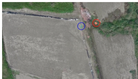
Figure 11. A red target board and a green agricultural net reported by the post-identification program, with both the red and blue targets marked with circles in corresponding colors.
