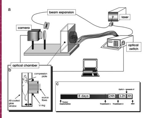
**Fig. 1.** The combined planar imaging/FMT system. (a) A schematic of the major components of the system is shown, with details given in the text. (b) Details of the imaging chamber that was used for planar, transillumination, and tomographic acquisitions of small animals. AR-coated, antireflection-coated. (c) Experimental protocol followed for the animal studies performed.
