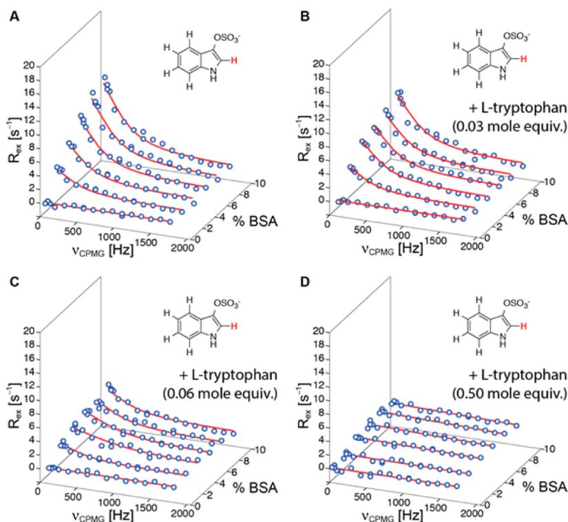
**Figure 3.** 500 MHz ligand-observed  $^1\text{H}$ -CPMG relaxation dispersion data for 2.0 mM indoxyl sulfate ( $^1\text{H}$ -2) interacting with BSA (up to 10% saturation) before (A) and after addition of (B) 0.06 mM (0.03 mol equiv with respect to indoxyl sulfate), (C) 0.12 mM (0.06 mol equivalents), and (D) 1.0 mM (0.50 mol equiv) of L-tryptophan.
