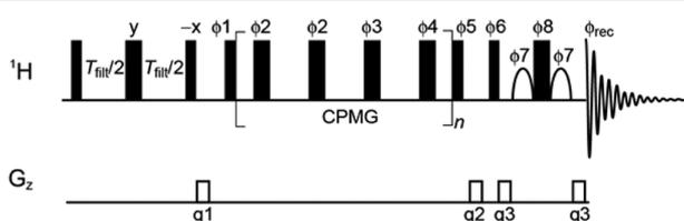
**Figure 1.** NMR pulse scheme for measuring ligand-observed  $^1\text{H}$ -CPMG relaxation dispersion profiles. During the CPMG element, pulses [ $\phi_2$ ,  $\phi_2$ ,  $\phi_3$ ,  $\phi_4$ ] are phase-cycled according to the [0013] alternation scheme.<sup>28</sup> See the [Supporting Information](#) for details.
