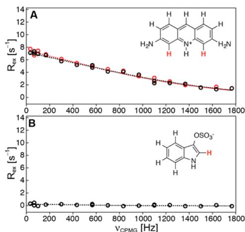
**Figure 4.** 500 MHz ligand-observed <sup>1</sup>H-CPMG relaxation dispersion data for (A) proflavin (<sup>1</sup>H-4/5) interacting with bovine trypsin (3% saturation) before (red) and after (black) addition of equimolar amounts of indoxyl sulfate and (B) data for indoxyl sulfate (<sup>1</sup>H-2) in the presence of trypsin (3% saturation).
