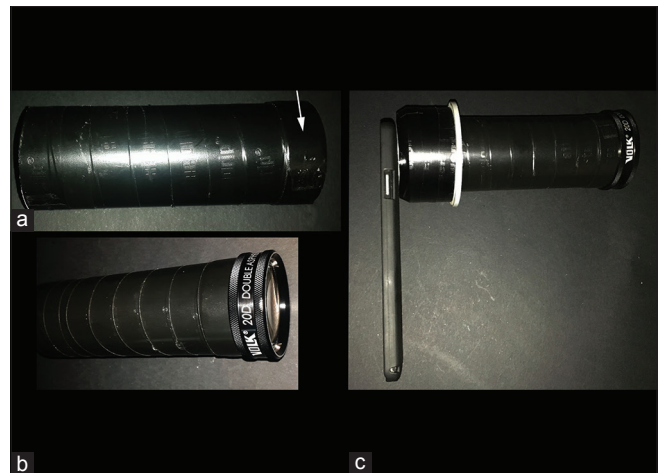
Figure 4: (a) The optical tube camouflaged with insulation tape. To fit the 20 D, few more rounds are applied to increase the thickness (arrow). (b) The condensing lens fixed on the optical tube. (c) The handheld device is ready to use
