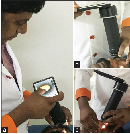
Figure 6: (a) The do it yourself smartphone fundus camera used as a hand held the device. (b) The do it yourself smartphone fundus camera can be held at the condensing lens and supported with the other hand on the camera. (c) Like in indirect ophthalmoscopy, scleral depression is done after stabilizing the do it yourself smartphone fundus camera
