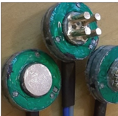
Figure 4: The final assembled active dry electrodes protected against the humidity and dust by silicon glue
