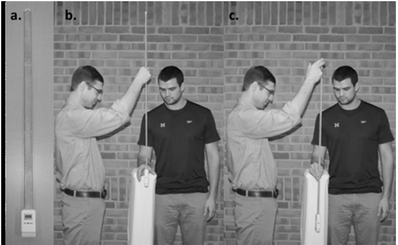
Figure 1. The Clinical Reaction Time Device (RT clin Dev) used to determine Simple RT clin Latency and Complex RT clin Accuracy.
