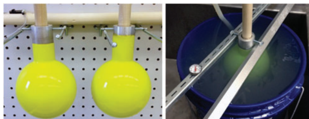
FIG. 5. Two freshly dipped mandrels hanging to dry (left). After dipping, dispersions are removed in a hot water bath (right). Color images available online at www.liebertpub.com/soro
