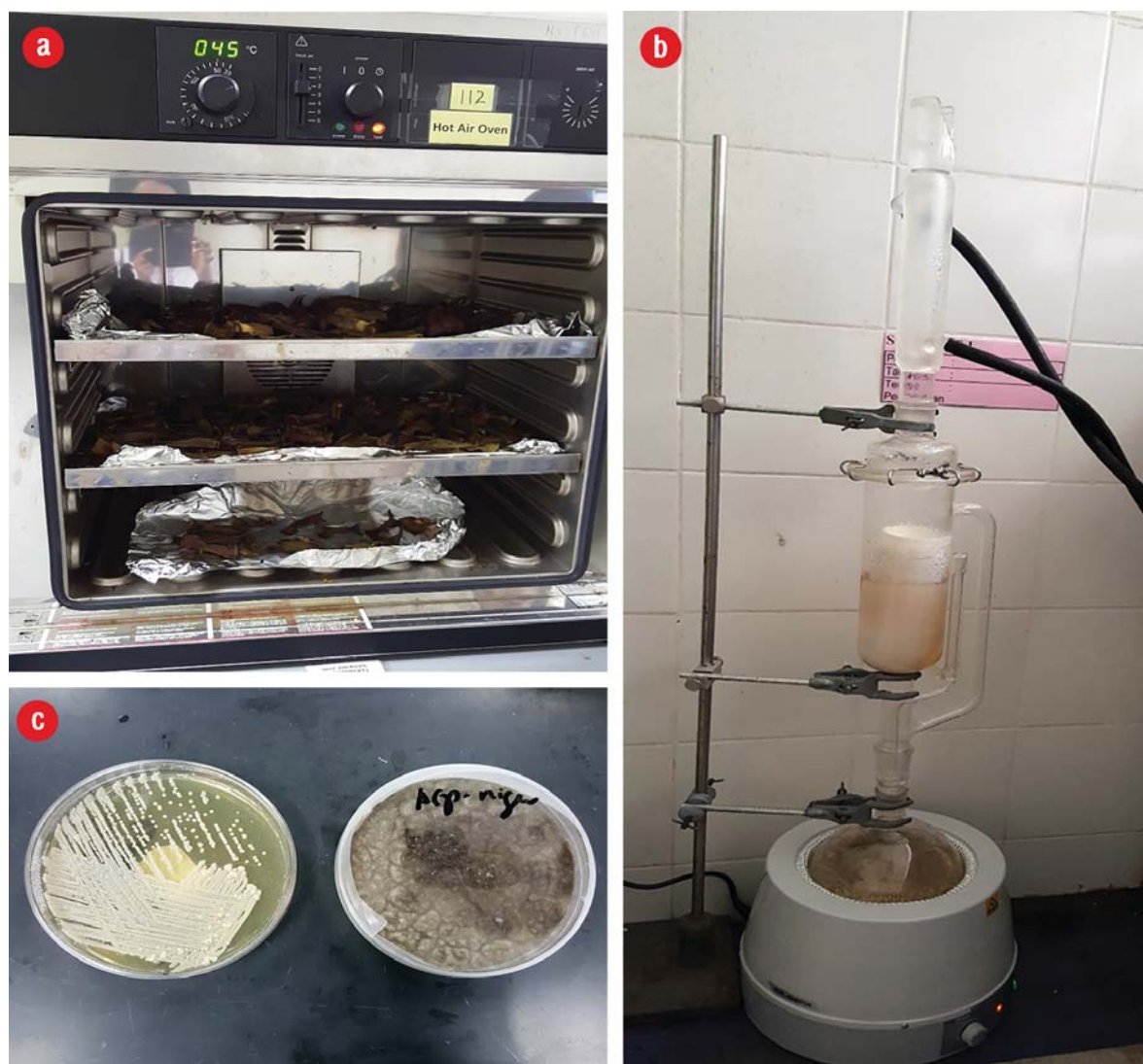
Figure 1: (a) Aloe vera leaves dried at 45 °C in a hot air oven. (b) Soxhlet apparatus used for extraction. (c) Candida albicans and Aspergillus niger culture.
