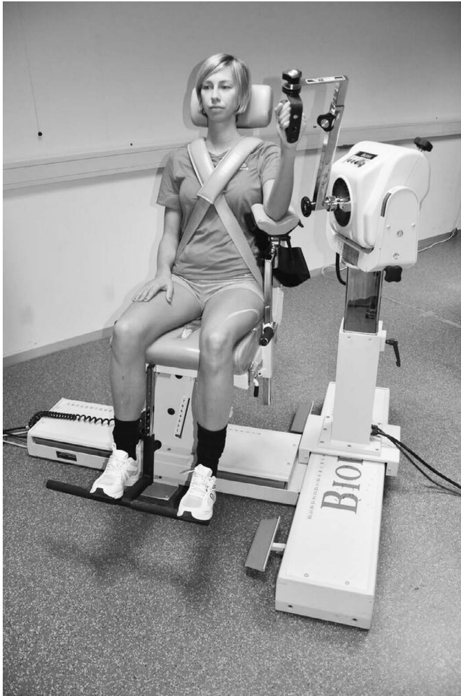
Figure 4. Setup for isokinetic elbow flexion and extension testing using an isokinetic dynamometer (system 4; Biodex Medical Systems Inc, Shirley, NY).
