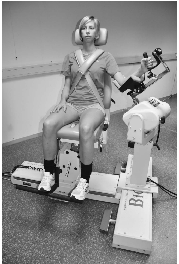
Figure 3. Setup for testing isokinetic shoulder external and internal rotation using an isokinetic dynamometer (system 4; Biodex Medical Systems Inc, Shirley, NY).
