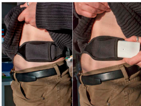
Figure 1. Image of the 9 \times 2 sensor and the neoprene belt.
