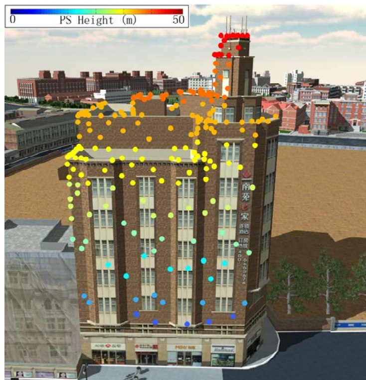
Figure 3. Three-dimensional representations of extracted Permanent Scatterer (PS) point geocoded on precise 3D models for the Bohai Building. All the PS satisfying the stability criteria during IPTA processing (sub-correlation coefficient larger than 0.35 and amplitude deviation measure larger than 1.4 ) have been located on roof and facades toward the satellite, in the monitoring period from May to December 2014.
