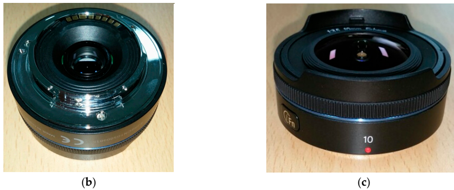
Figure 3. (a) Optical layout of the optimized fisheye lens system and (b) top and (c) bottom views of the fabricated fisheye lens system.
