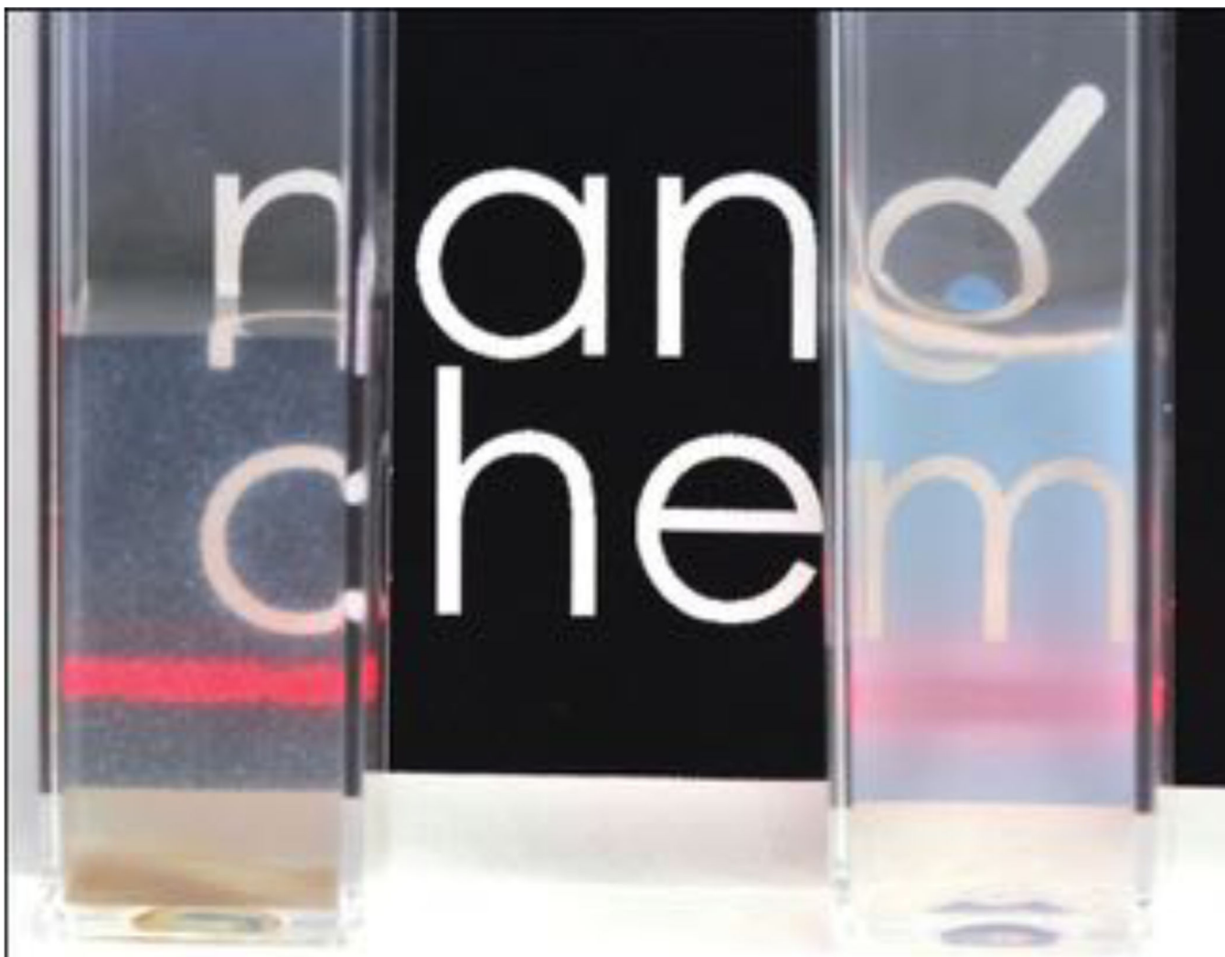
Figure 4. Photography of \text{ND}_1 and \text{ND}_4 dispersions ( 0.5 \text{ mg mL}^{-1} ) in PBS, 30 min after mixing. \text{ND}_1 (left) precipitates and finally gives sediment at the bottom of the tube, while \text{ND}_4 (right) remains in the form of stable colloid scattering the laser beam (red laser pointer).
