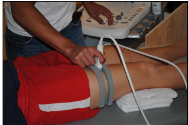
Figure 4. The high-density foam served as a guide for the sound head, thus minimizing tilt and rotation.
