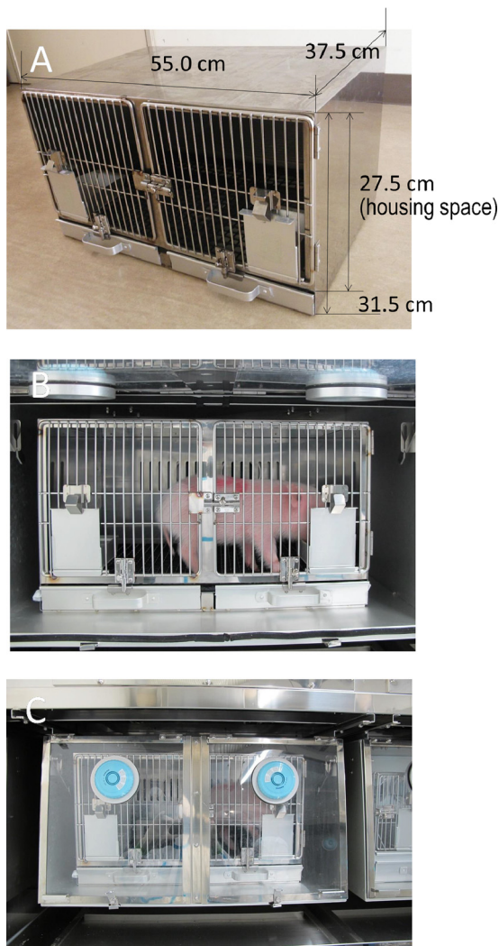
FIG 1 Images of the cage and the isolator. (A) New isolation cage produced for this study of 8- to 12-week-old microminipigs. (B) Negative-pressured isolator containing the isolation cage with a micro-minipig (1.46 kg) inside. (C) Negative-pressured isolator with a hatch door with HEPA filters (blue and round) closed.
