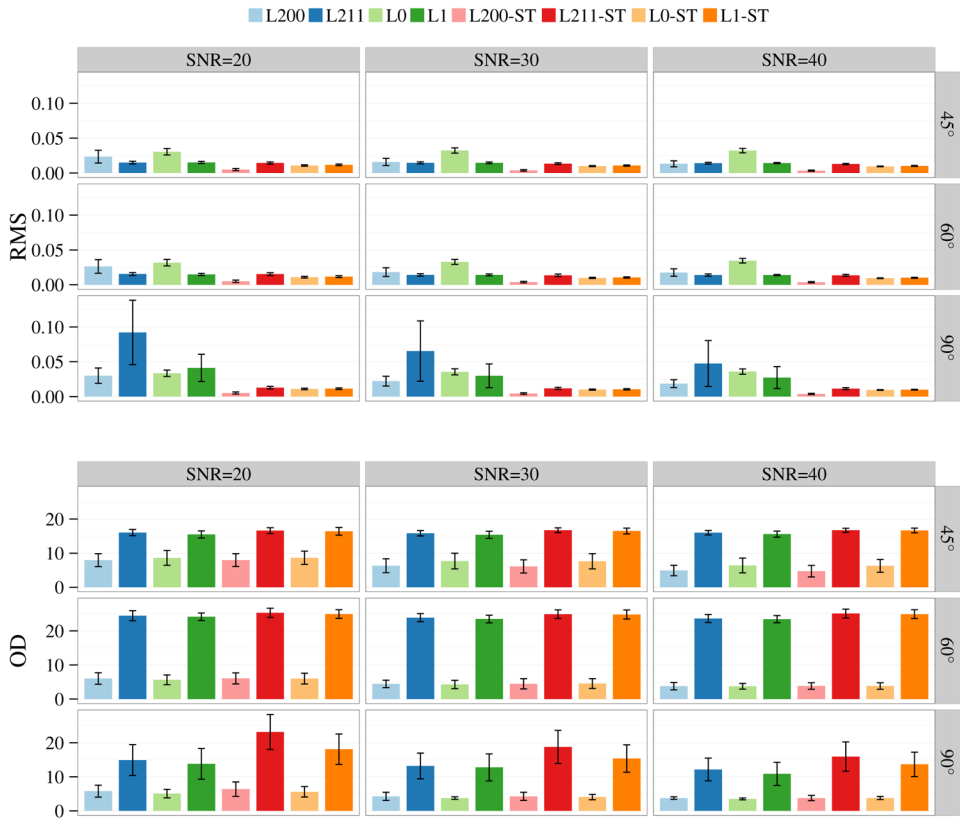
Fig. 3. Estimation accuracy for volume fractions in terms of RMS error and FODFs in terms of OD. Only the WM compartments were used to generate the data. The bar plots show the mean performance statistics for SNR = 20, 30, 40 and crossing angle = 45°, 60°, 90°. The error bars indicate the standard deviations.
