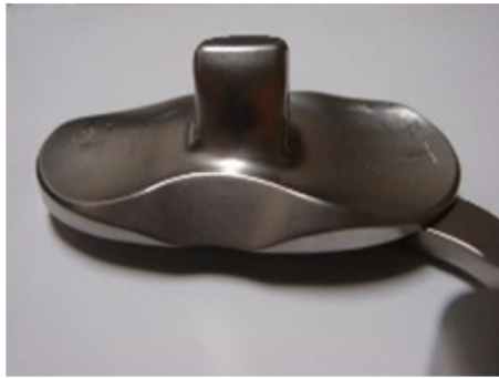
Fig. 4. Photographs showing the new tensor. The upper plate has identical shape as polyethylene surface trial (size: 9) of Journey. 2. BCS.
