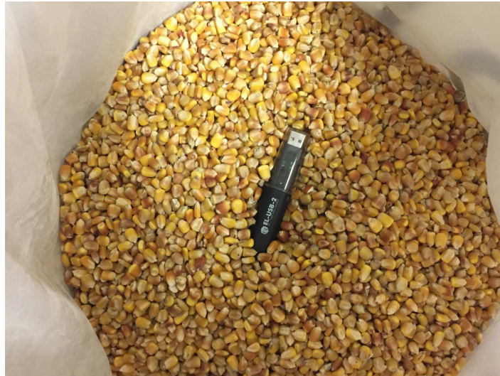
Fig 1. Data logger as seen before sealing of the PICS bag. Wireless data loggers were used to measure temperature and relative humidity conditions within PICS bags. Data loggers were pushed into the center of the maize bulk prior to sealing the bags.
