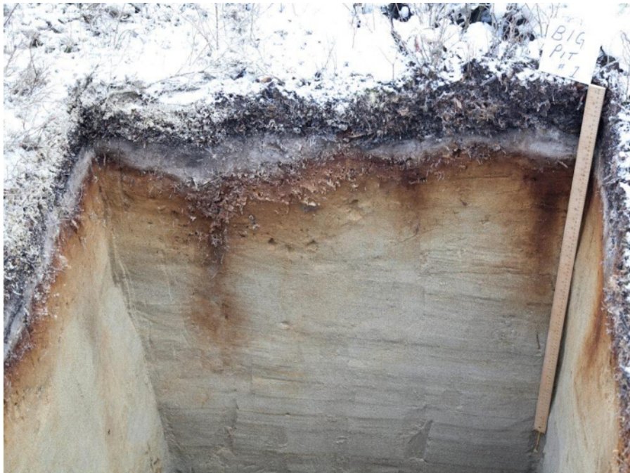
Figure 5: Example of horizon expression. A soil profile with horizon boundaries that have distinctness classes of clear or gradual and topography that is wavy or irregular. Please click here to view a larger version of this figure.
