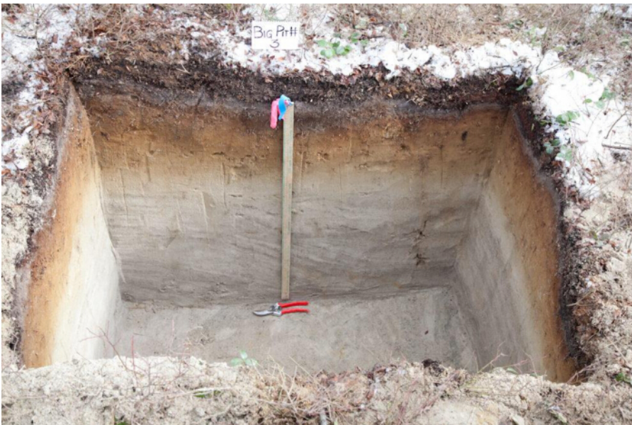
Figure 4: Example of horizon expression. A soil profile with horizon boundaries that have distinctness classes of abrupt or clear and topography that is smooth or wavy. Please click here to view a larger version of this figure.
