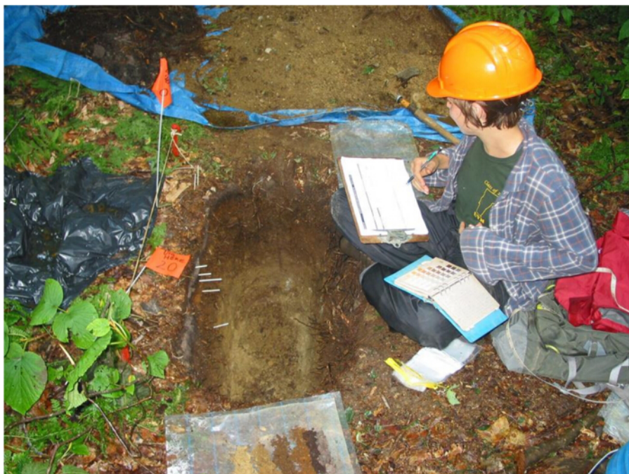
Figure 2: Completed pit excavation. Soil pit excavation showing the removed mineral soil and intact forest floor on a tarp to minimize site disturbance, along with pins marking horizons on the pit face. Please click here to view a larger version of this figure.
