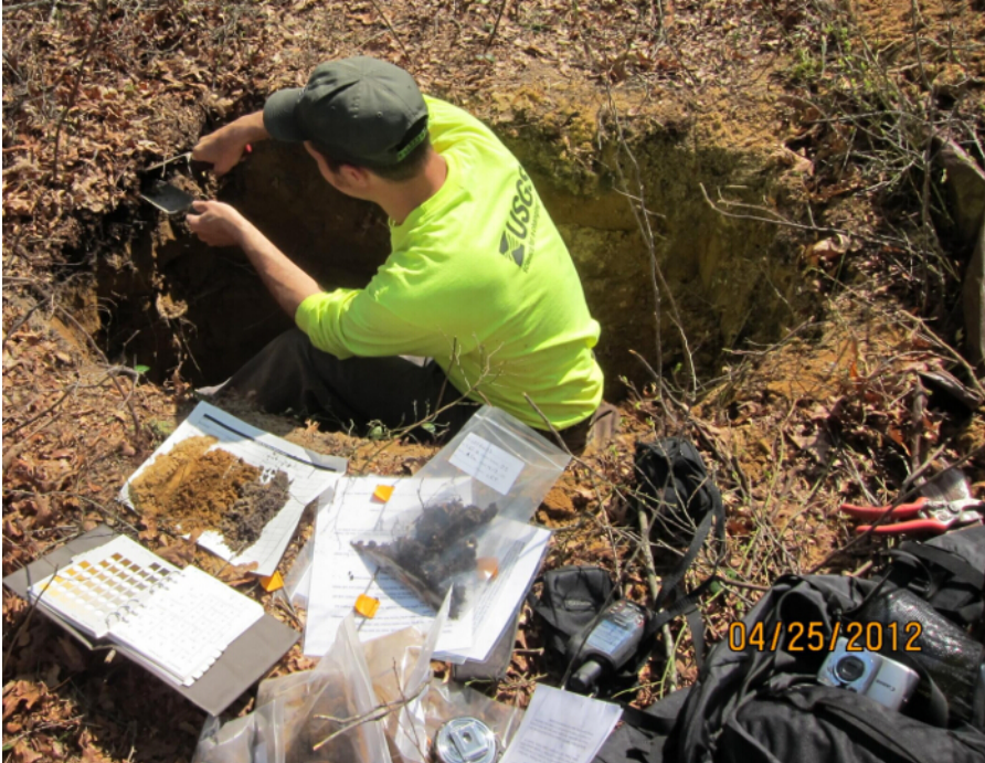
Figure 3: Sample removal technique. Technique used to remove soil from the pit face. Also shown are samples of differing colors removed from the pit face, aligned in order, to help identify horizon boundaries. Please click here to view a larger version of this figure.
