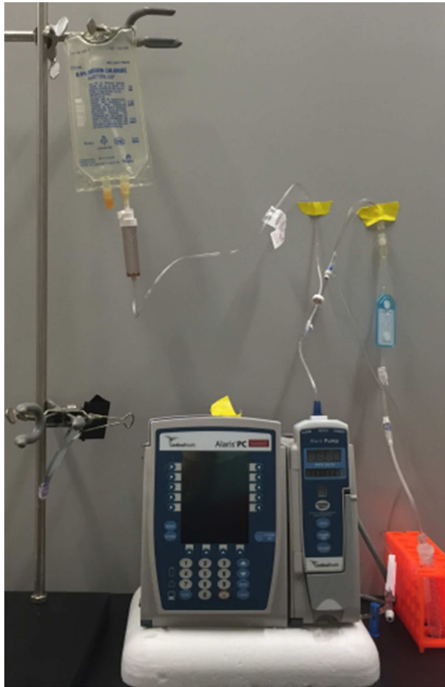
Figure 1. Setup in the lab replicating a typical IV infusion system used at the Outpatient Infusion Center at the University of Colorado Hospital
