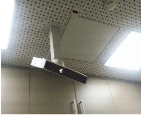
(a) One of two camera-projector units of AlignRT (optical sensor) at the ceiling in treatment room. It consists of a stereo camera and a projector producing structured light by laser speckle in a fixed arrangement
