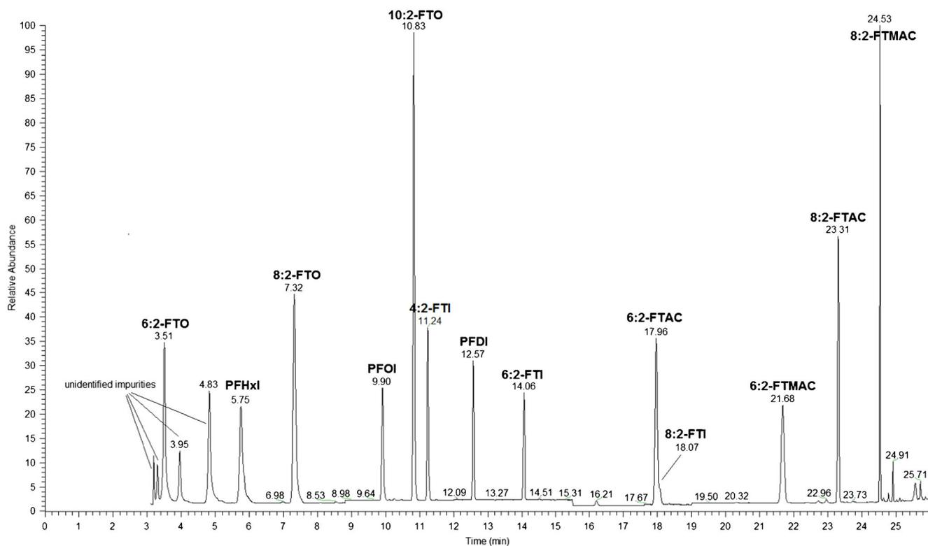
**Fig. 4** Total ion chromatogram of 600 ng/mL standard solution determined by +EIMS (70 eV electron energy) in SIM mode
