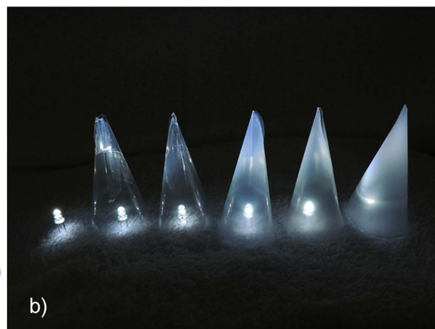
Figure 7. Total light transmittance and haze value of nanopaper (a), and the application of hazy transparent nanopaper as optical diffusers (b). Far left: an LED light without diffuser, from second-to-left to right: increasing nanopaper haze, which homogeneously spreads the light through the nanopaper and maintains light intensity.
