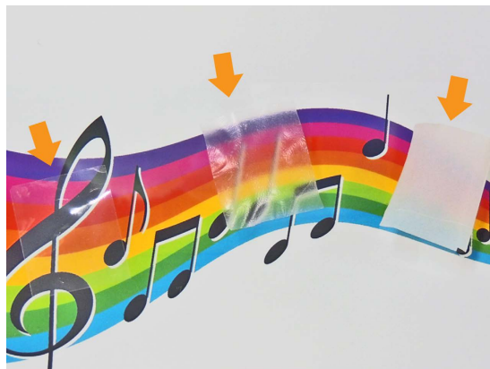
Figure 1. Various appearances of cellulose nanopaper consisting of 15-nm-wide nanofibers. Left: Clear transparent nanopaper with a density of 1.48\text{ g/cm}^3 . Center: Translucent nanopaper with a density of 1.15\text{ g/cm}^3 . Right: Opaque nanopaper with a density of 0.81\text{ g/cm}^3 .
