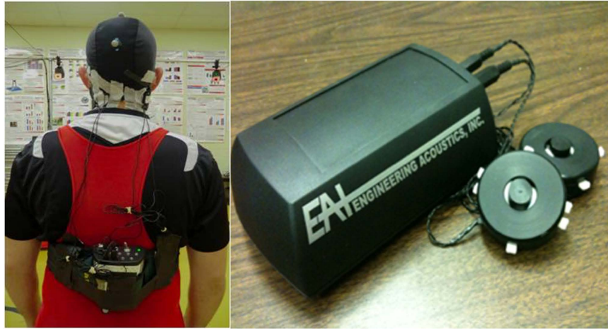
Figure 4. The tactor system contains two tactors and a controller unit for communication with the computer through Bluetooth and transmission of stimulus control signals to the tactors.
