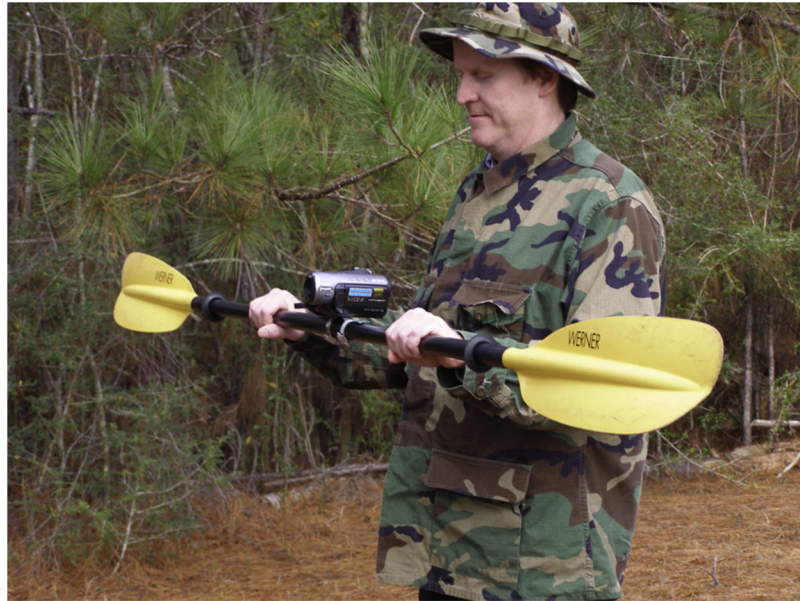
Fig. 1. High-definition video camera mounted on kayak paddles used in this study. The focus is set to a moderate range (such as 50 m), and the camera is kept recording at all times. With this set up, the paddles may be used to get the camera on a bird almost instantly as illustrated in the example in Movie S2.
