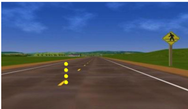
Figure 1. Illustration of LDW visuals (bottom) and the subject's corresponding lane position (top)
