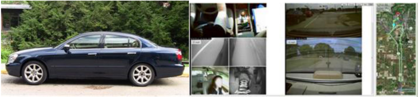
Figure 2. Views of the instrumented vehicle for standard on-road drives.
