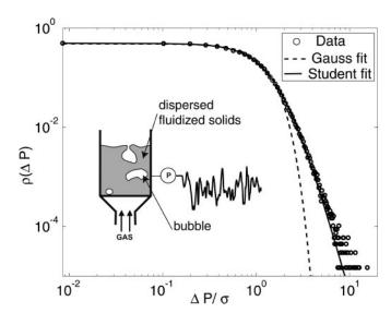
Fig. 4. Student's (solid) and Gaussian (dashed) fit of the PDF of pressure fluctuations in a gas-fluidized bed of solid particles. Pressure increments  $\Delta P = P(t+\Delta t) - P(t)$  over a time interval  $\Delta t = 50$  ms are normalized to their standard deviation  $\sigma$ . The Student fit yields  $n \approx 3$ . (*Inset*) Sketch of the pressure measurement (see ref. 18 for complete details).
