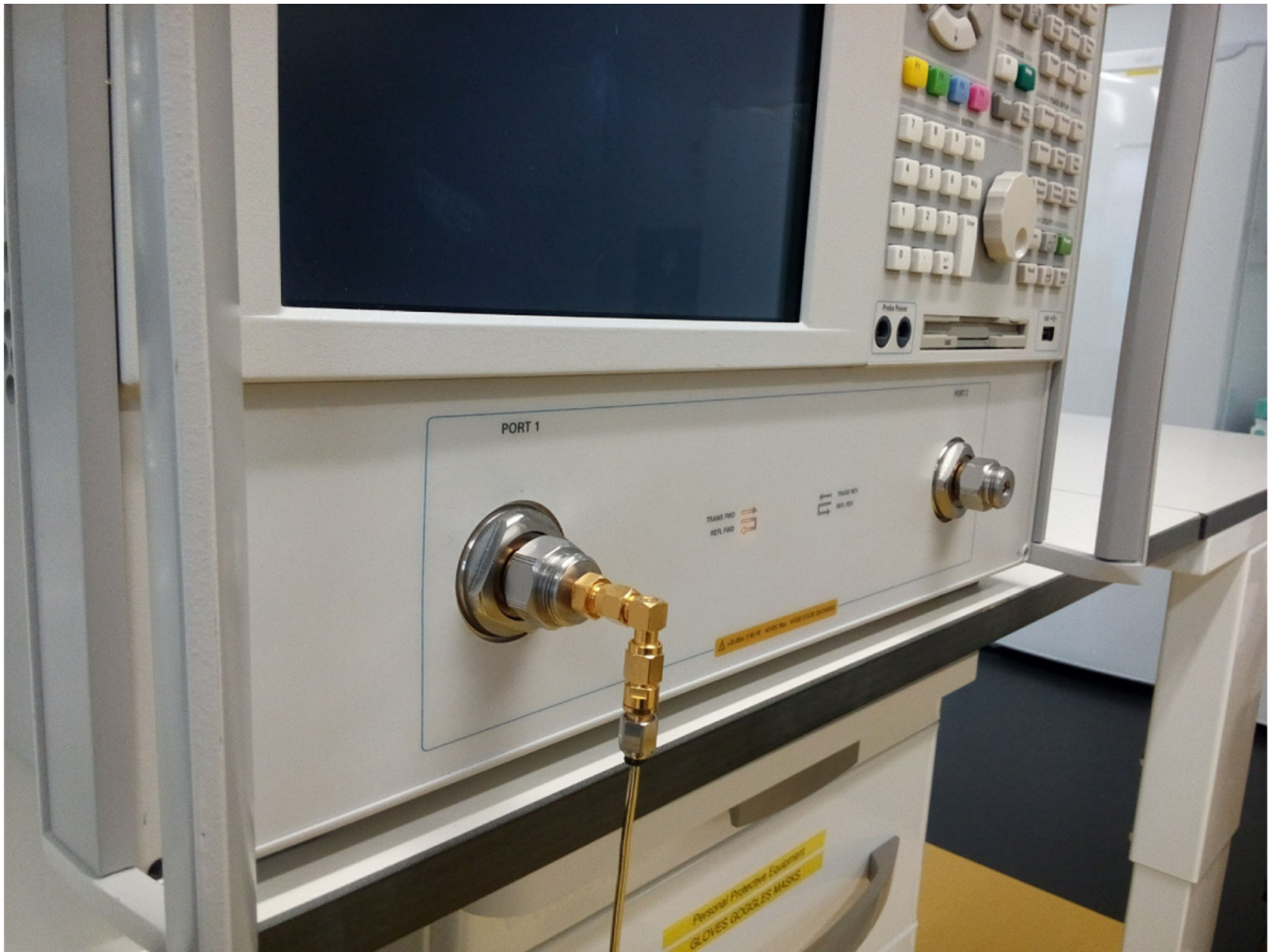
Fig. 1. Photograph of the slim form probe connection with the network analyser.
