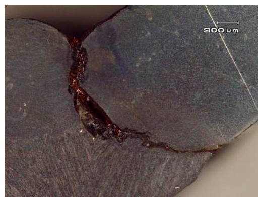
Figure 1. Lack of fusion and crack defects of welding.
