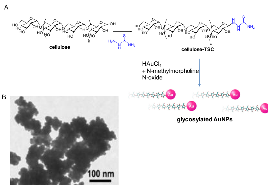
Figure 4. Synthesis of glycosylated AuNPs. (A) Synthetic scheme; (B) TEM image of glyco-AuNPs.
