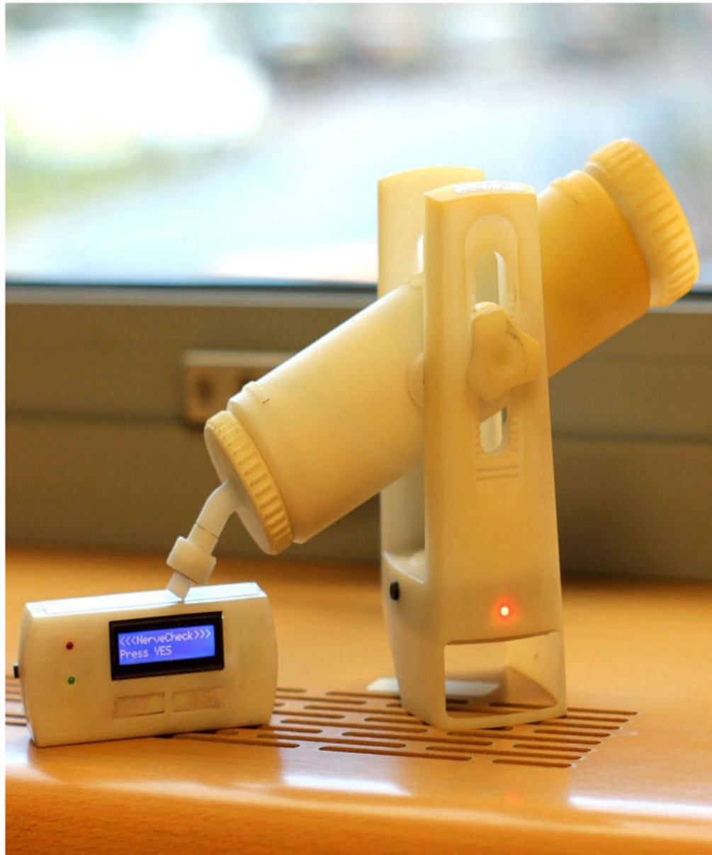
Figure 1. NerveCheck is a portable inexpensive ($500) quantitative sensory device designed to assess vibration (VPT), cold (CPT), warm (WPT) perception threshold and heat pain threshold (HPT). Its size is 9.5 cm × 6.1 cm × 23.6 cm and weights only 325 g, including battery. Its output is categorical in terms of degree of abnormality. The test takes from 3–10 min, depending on whether it is a single test or series of tests.
