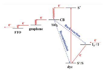
**Figure 5.** Schematic diagrams of the energy levels in the reduced graphene oxide-CdSe based quantum dot sensitized solar cell [60]. Reprinted with copyright permission from [108]. Copyright © 2011, American Institute of Physics.
