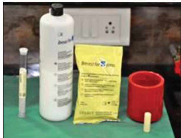
Figure 3: Bresol investment liquid and investment material
