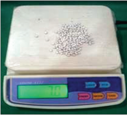
Figure 4: Seven grams of polyetheretherketone dental material
