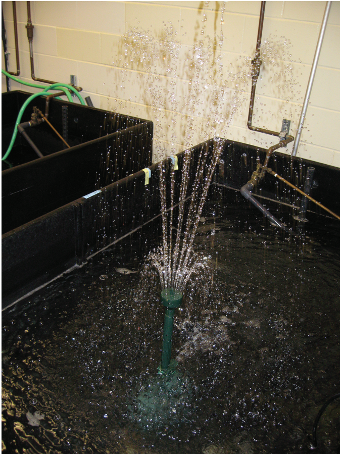
Figure 10. The supersaturated water was aerated by installing fountain heads (Little Giant, Oklahoma City, OK), which increased the air–water interface to enhance the transfer of dissolved gases in the water to the atmosphere.
