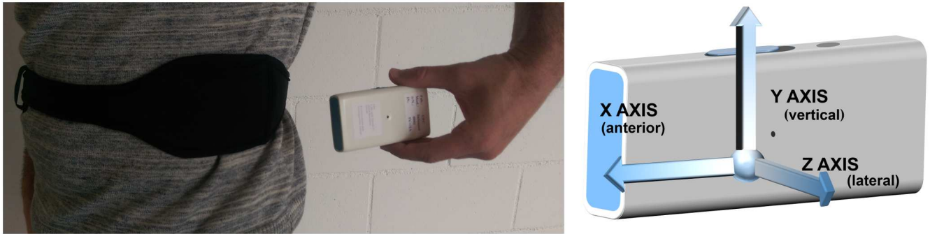
Fig 2. The 9x2 and location of the IMU.
