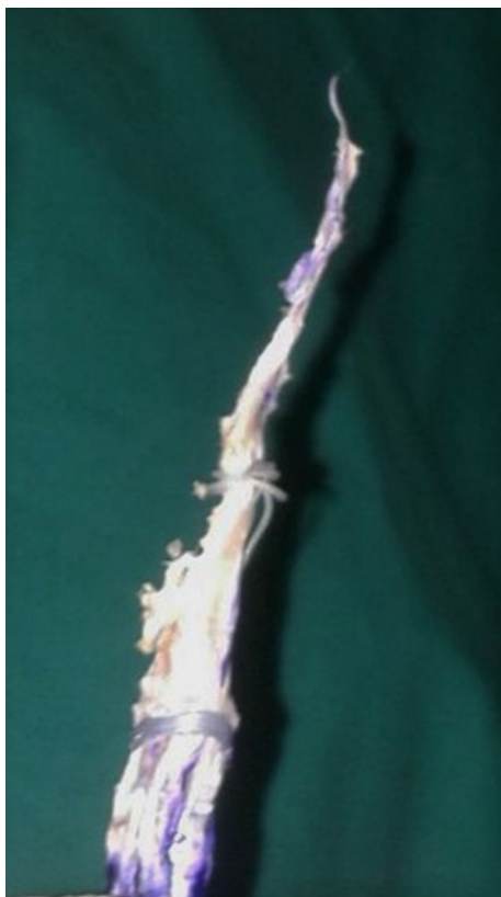
Fig. 6 Mode of failure: tendon slippage across the suture (“tripled” configuration)
