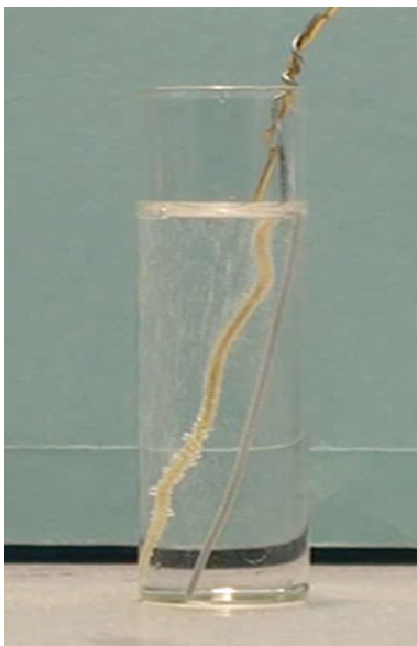
Figure 7. Wollaston's experiment, with zinc and gold wires.
