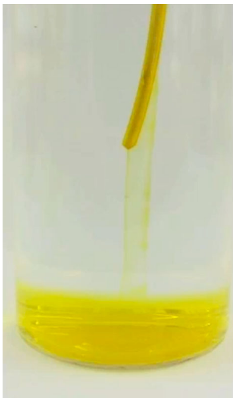
Figure 9. The dissolution of a gold electrode in salt water.
