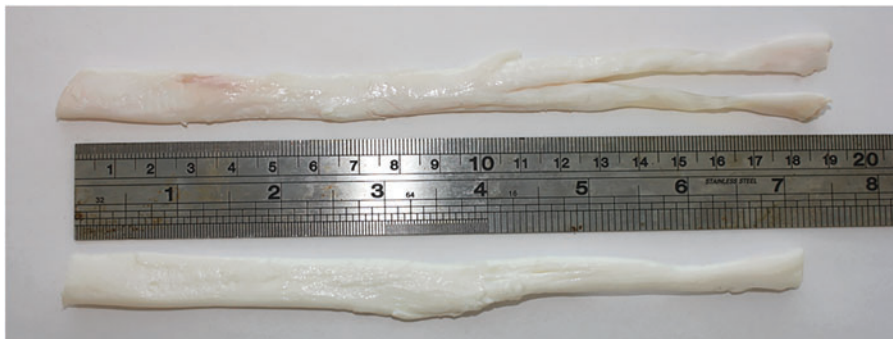
FIG. 1. Image of the porcine superficial flexor tendon (SFT) before ( top ) and after ( bottom ) decellularization.
