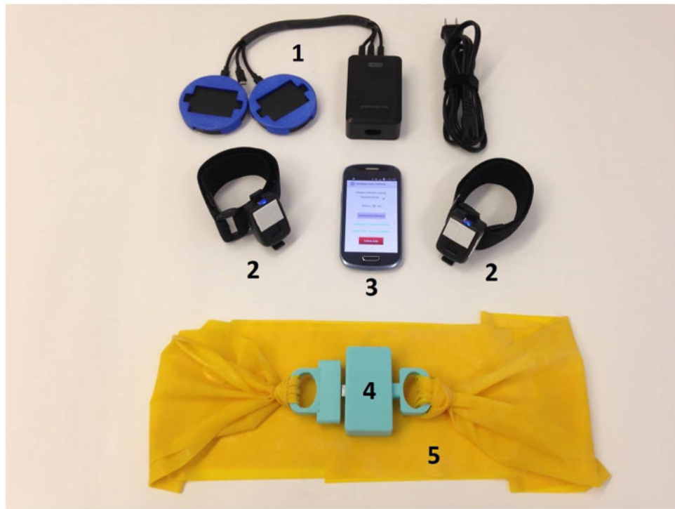
Figure. Components of a Rehabilitation-Internet-of-Things: wireless chargers for sensors (1), ankle accelerometers with gyroscopes (2) and Android phone (3) to monitor walking and cycling, and a force sensor (4) in line with a stretch band (5) to monitor resistance exercises.
