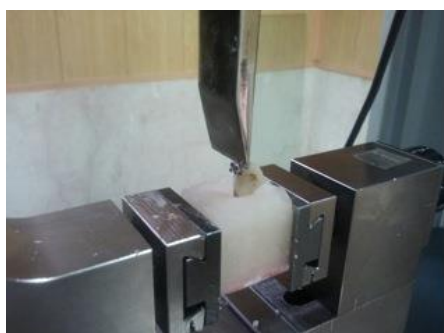
Fig. 1: Testing shear bond strength of metal brackets
