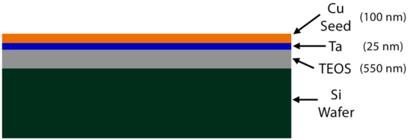
Figure 1. A cross-sectional illustration of the substrate before copper electroplating.
