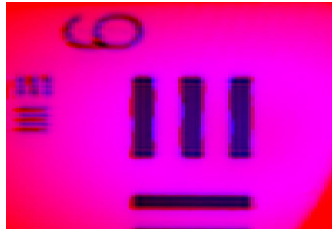
Fig. 2. Co-registered images (150 x 100 \mu\text{m} ) of a Group 6, Element 1 of a USAF-1951 resolution target acquired from the fluorescence (blue) and OCT (red) imaging systems.
