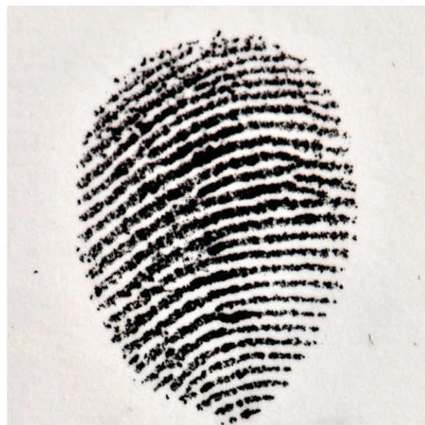
Figure 4. A typical fingerprint image obtained at a normal force of 2 N for a finger pad orientation of 45^\circ .
