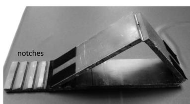
**Fig. 1.** Two boards that were each 68 cm long and 13 cm wide and that could be combined to form a wedge were designed. A movable joint was included between the two boards. Another movable joint was included on the upper board, such that one side was 38 cm long and the other was 30 cm long.
