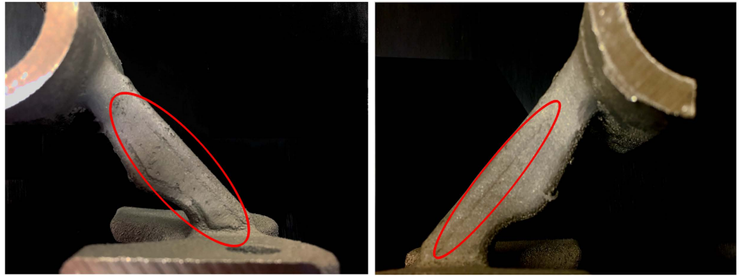
Figure 18. Images taken of the part after the build was completed. Surface swelling (right) and pitting (left) can clearly be seen in the part and could be a potential causes of algorithm failure.
