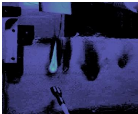
Figure 7. Flames erupting from the GF composite at t \approx 30 s during a direct laser strike on the sensor at position 4. The N_2 nozzle can be seen just below the flame.
